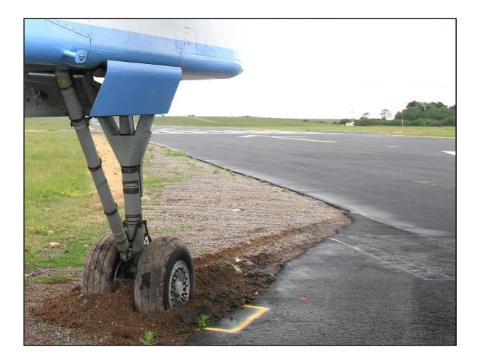
**Photo No. 1:** Embedded right hand wheels with RWY 21 threshold in background.
